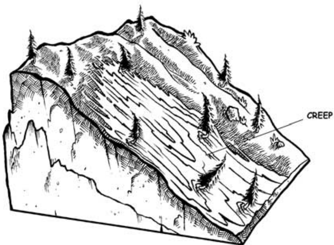
Figure 11. Soil creep and earth flows occur as gravity moves soil downhill toward streams. Trees on the surface of an earth flow often become tilted as the soil they are rooted in moves downhill.
