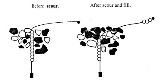
Scour during peak flows occurred on all cross-sections in all habitat types. The average depth of scour for all cross-section monitors was 0. **1**  $\mathbf{n}$  (range 0.0-0.6 m). The average depth of scour in Reach B (0. **14** m) was nearly double that of Reach A (0.8 m). Scour at 19.7% of the monitors reached a depth of 0.2 **m**, the median depth of chum **salmon** egg pockets (Chapter I-A). Scour at 27.9% of the monitors in Reach B reached 0.2 **m**, compared to only 9.1% in Reach A.
