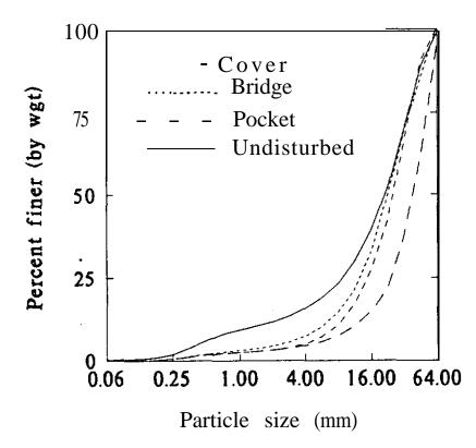
Figure I-A- $\sim$ . Cumulative distribution (combined sample dry weights) for 29 egg pockets in the spring.
