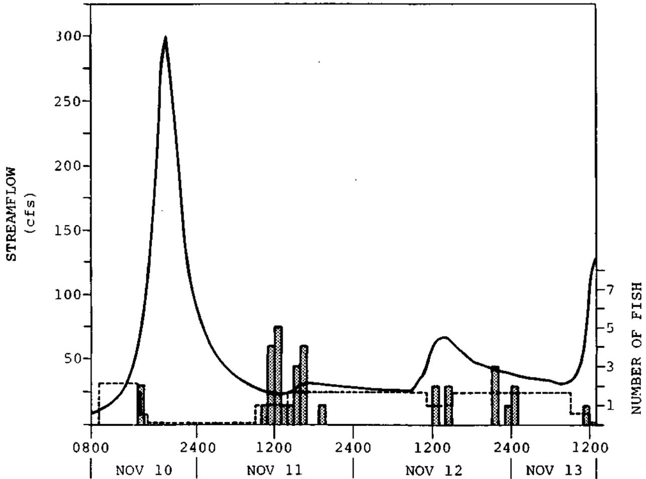
Figure 3-2. Hourly streamflow measured at the SPTSP gage (solid line), number of coho salmon observed migrating upstream (histograms), and release from Kent Lake (dashed line) in Lagunitas Creek, November 10-13, 1983. Fish observations were continuous except between 1900 hrs on November 10 through 0800 hrs November 11 due to high streamflow and turbidity.
