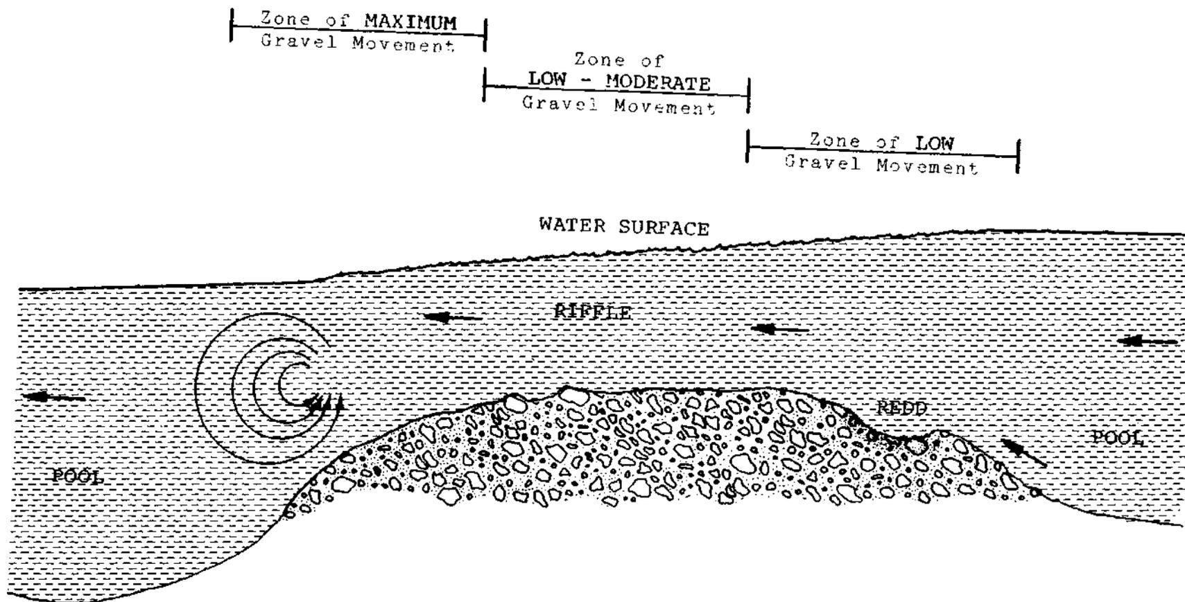
Figure 4-4. Zones of gravel stability for a typical riffle (from Yee 1984). For redd building, coho salmon almost always selected the upstream portion of the riffle, where the risk of scour is lowest.
