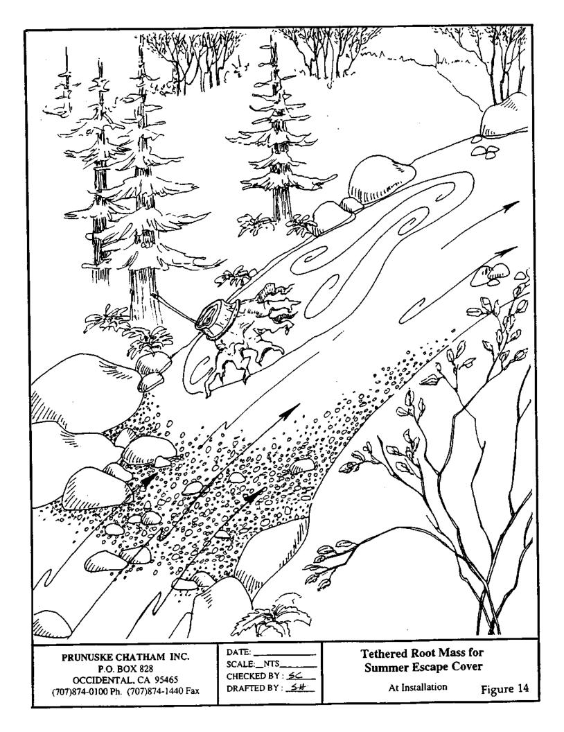
channel double log structure (Figures 7 and 8), the single oblique obstruction log (Figures 9 and 10), the double oblique obstruction log (Figure 11), tethered tree tops (Figure 12), tethered logs (Figure 13), and tethered root mass (Figure 14). The amount of this type of woody debris that is needed is governed by the number of pools in the system that are escape cover deficient.
