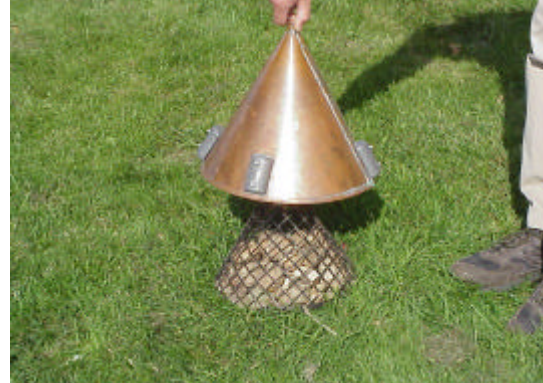
Figs. 8-9. Remote-retrievable rock-filled cone and retrieval funnel for sampling non-wadeable rivers
