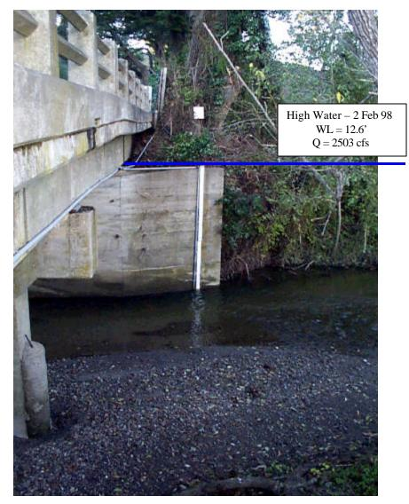
that two sets of rating curves are necessary. One curve is used when the flow covers only one-half of the channel bottom. The other curve is used once flow extends to both sides of the bridge abutment. After large events, the channel bottom changes, so flow measurements should be concentrated on these events.
