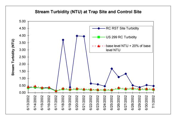
Figure 12. Comparison of stream turbidity above and below Chezum Dam, 2002.
