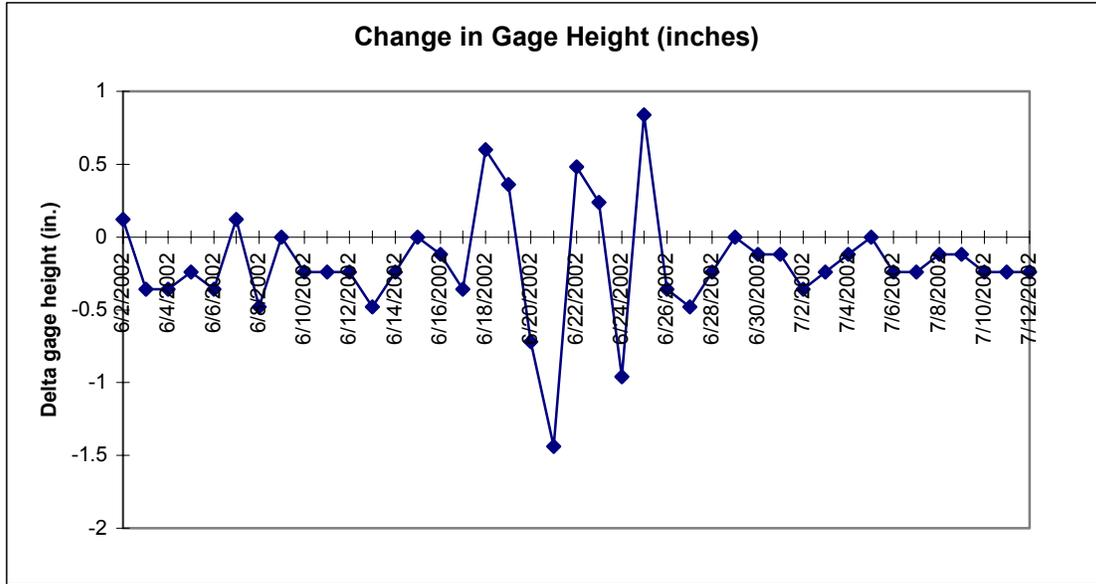
Figure 11. Change in gage height (in.) at the trap site during Chezum Dam operations, 2002.
