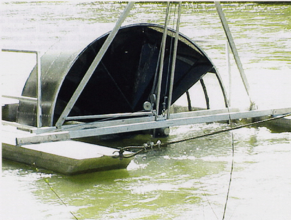
Figure 3-2. Rotary screw traps (under relatively high flow conditions) in the Russian River below the Inflatable Dam.
