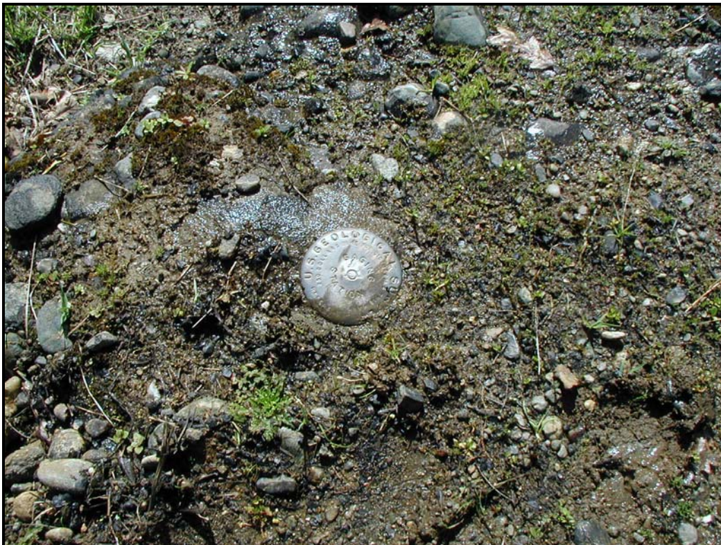
USGS Reference Mark near the Hayfork Creek in Hyampom Gage.
