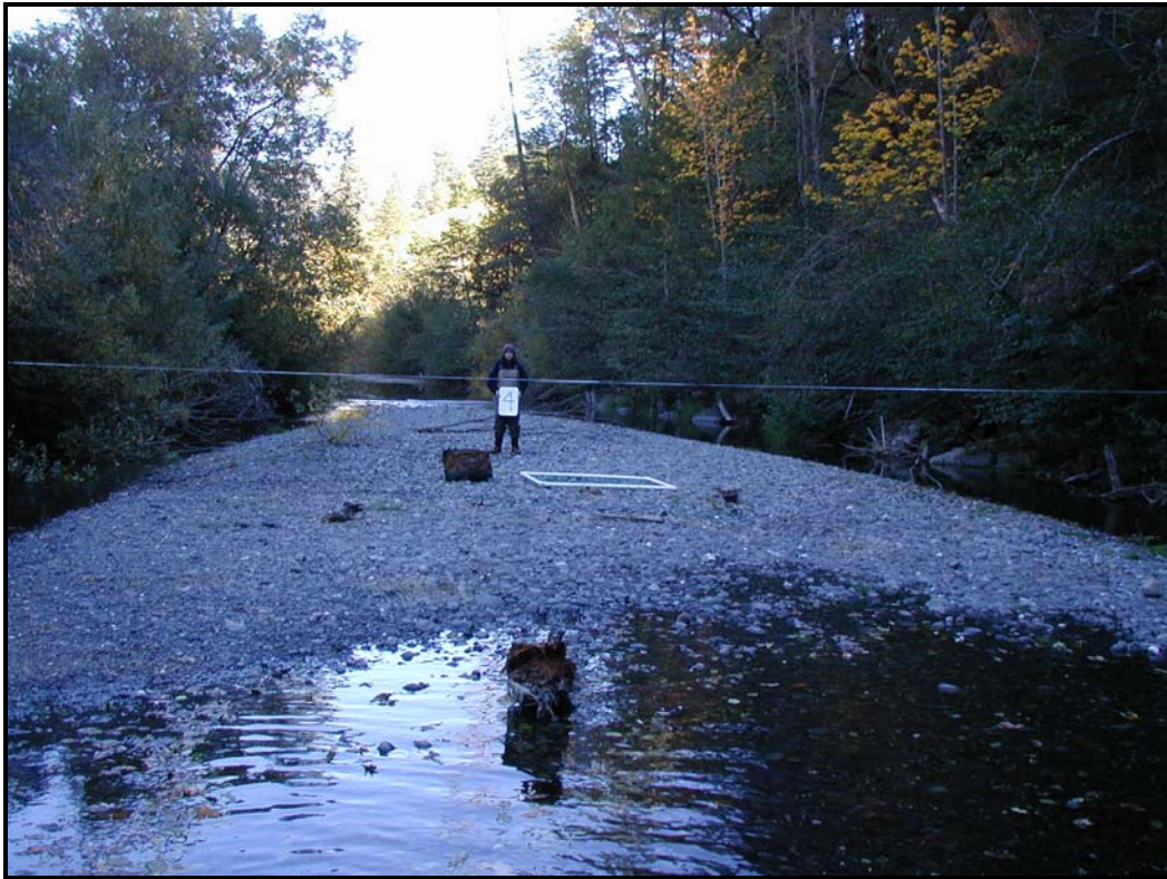
Pebble count sampling grid on Grouse Creek mid-channel bar, Cross Section 4.
