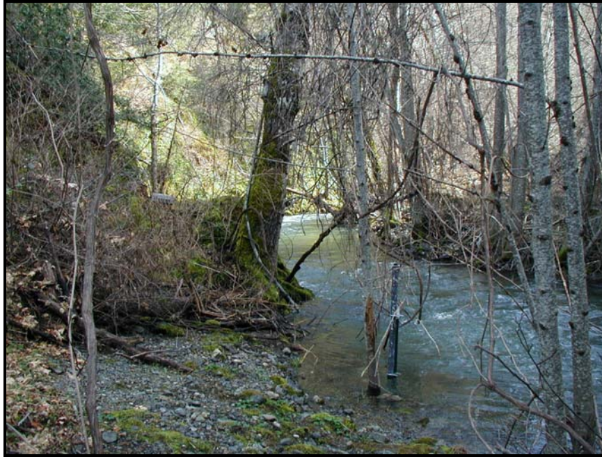
Steel gage house contour-mounted to downstream side of tree on Eltapom Creek.
