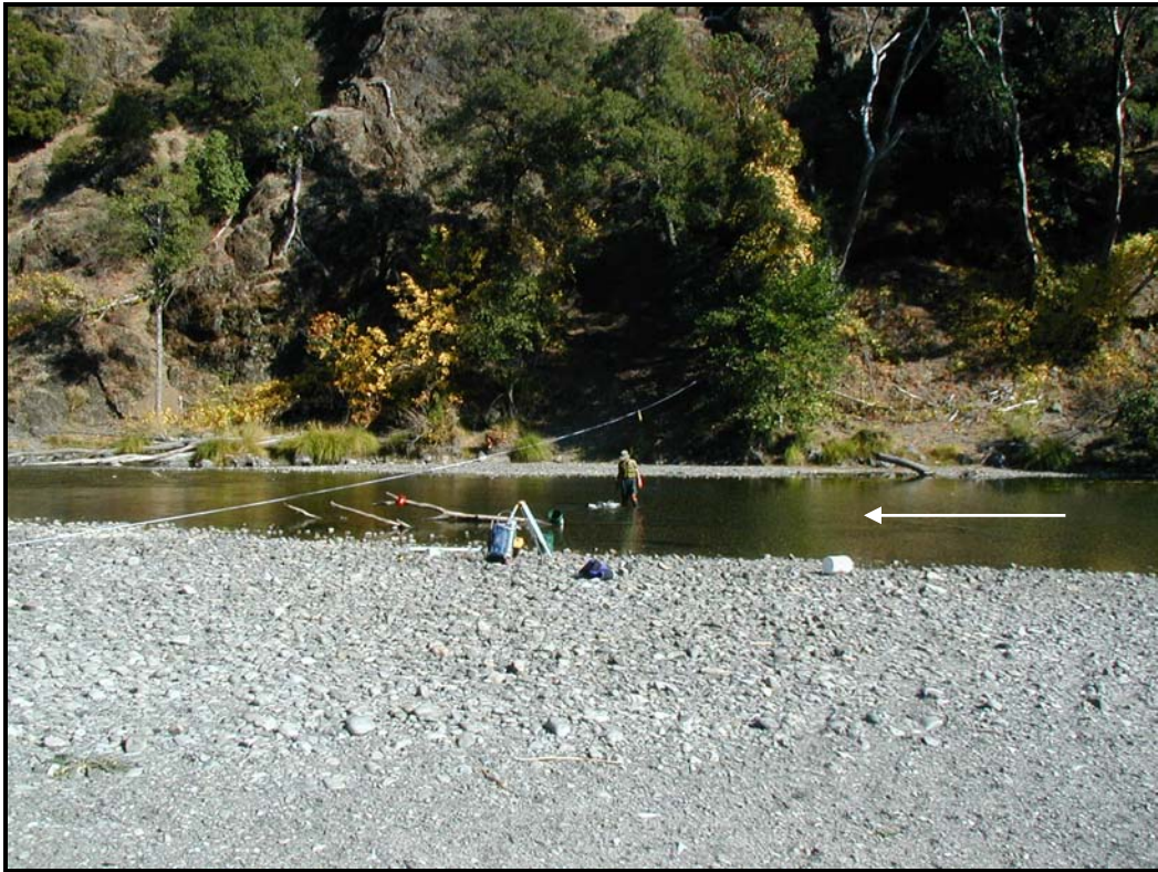
Bulk sampling of mainstem spawning gravels along a surveyed cross section (SFTEC).
