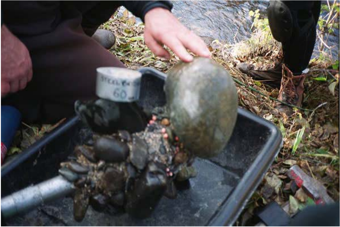
Figure 20. Photograph of core sample with large diameter cobble, Trinity River, California (Fall 2000).
