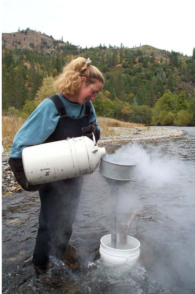
Figure 5. Photograph of the freeze-coring process; liquid nitrogen is being poured into a standpipe to freeze a sample of the substrate.
