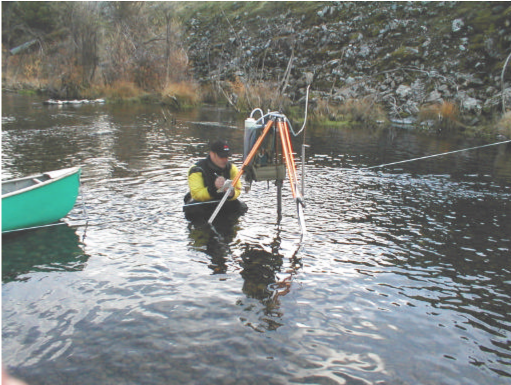
Figure 3. Permeability sampling using the backpack pump mounted on a tripod.
