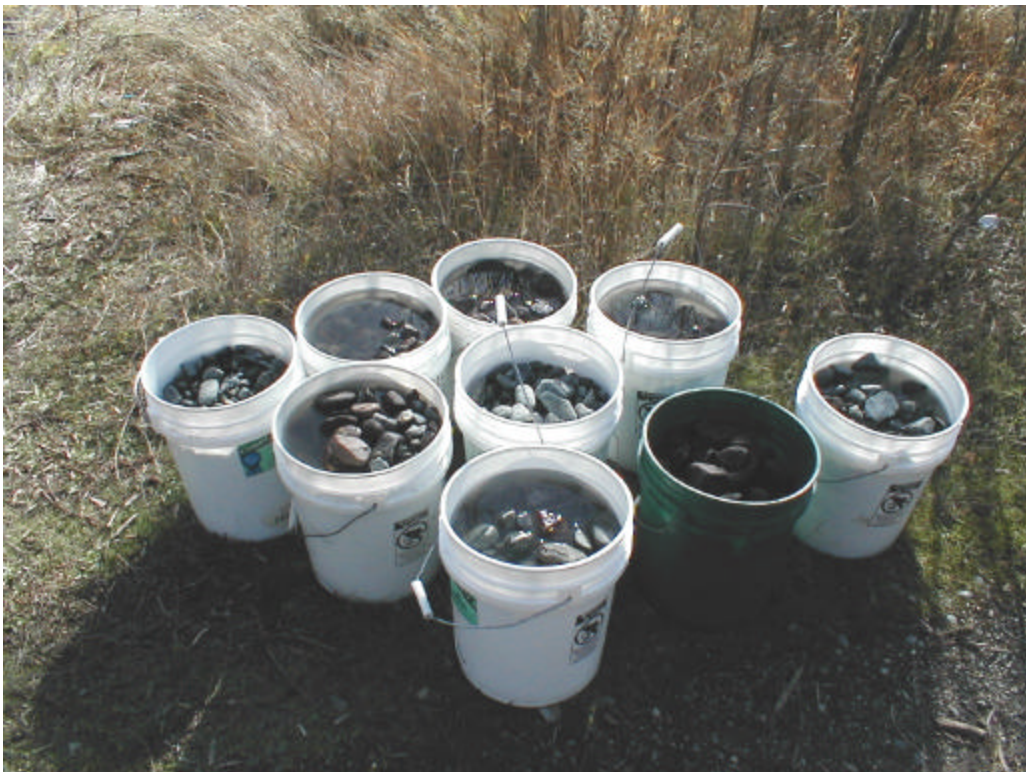
Figure 6. One bulk sample ready for field sieving. Note green bucket with surface sample.
