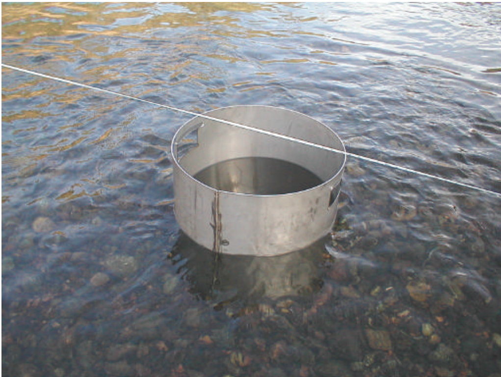
Figure 4. Two foot diameter McNeil type bulk sampler.
