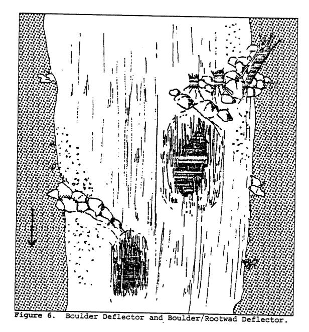
Boulder Deflector and Boulder/Rootwad Deflectors are small bankside structures (Figure 6) placed in riffle or run habitats to encourage channel deepening and habitat diversification. These structures were placed in the South Fork Salmon River and The East Fork of South Fork Salmon. The objective of structure placement was to provide rearing habitat adjacent to the structure (high velocity scour pool habitat) and stable spawning habitat on the upstream edge of the structure.
