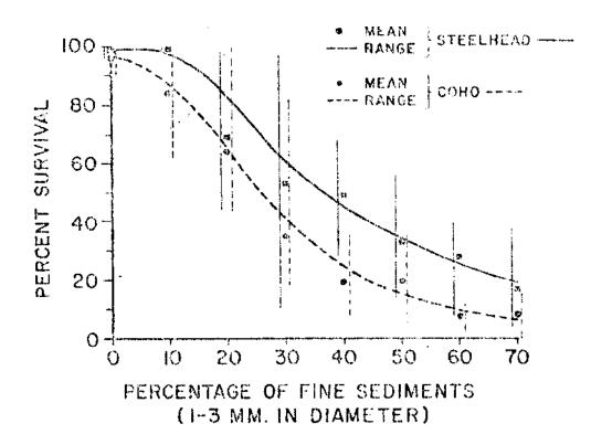
Figure 3. The relation between percentage of fine particles in an artificial gravel bed and the ability of Coho salmon and steelhead trout fry to emerge through the gravel.
