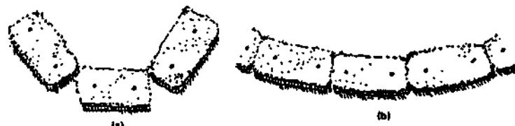
(a) Incorrect and (b) correct abutment of straw bales in a trench.
